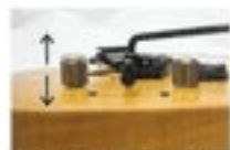
Master Tone with Bridge and Neck Pickup Coil Split Switch
