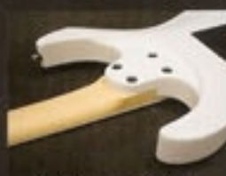
Neck Joint and Heel Cut
