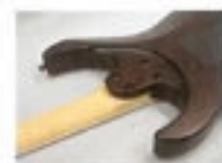
Neck Joint and Heel Cut
